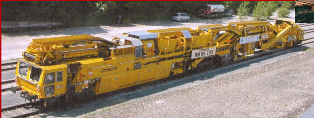
RM 95 - 700 /Ballast Cleaning Machine
